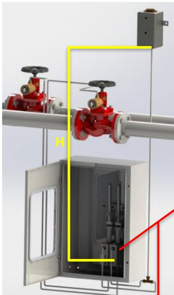
System is not activated, lever is fixed by compression latch.
