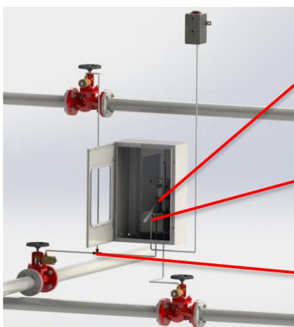
The lever has been engaged and the working piston has pressed down more oil into pipes system. Activation of connected cylinders is done and valves auto shut.
