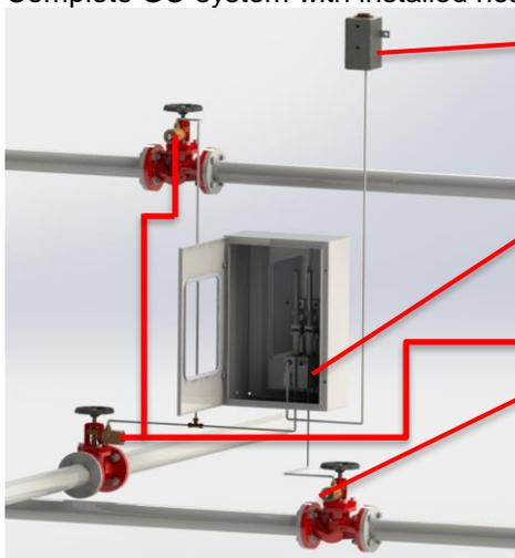
Header tank is installed at the highest point and serves all the installed pipes with oil and correct system levelling.
