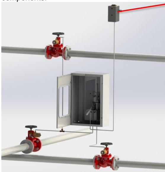
GC-header tank with an oil reservoir acts as the leveller
