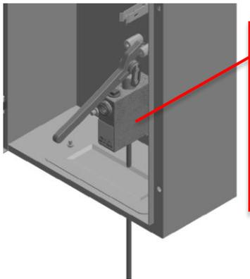
Active force on the working piston, connection between oil reservoir and working pressure chamber has been cut off.
