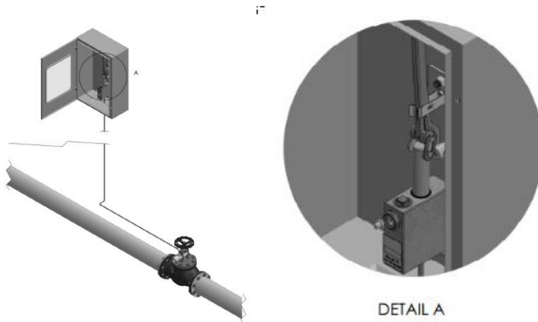
Lever is not activated, it is locked in position by compression latch.
