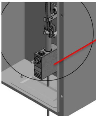
No active force on the working piston, connection between oil reservoir and working pressure chamber gives the same pressure in complete hydraulic system and complete system is vented through ventilation cavity on oil reservoir.
