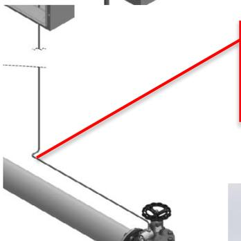
Depending on the height difference between the reservoir and the piping system the static pressure in the system will fluctuate depending on the height from the reference (<http://hyperphysics.phy-astr.gsu.edu/hbase/pflu.html> )
