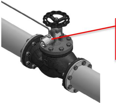
Release cylinder, rated operating PN30, rated static pressure 4bar. The 4 bar static pressure is to accommodate the static pressure that builds up due to the height from the GC-lever oil reservoir.
